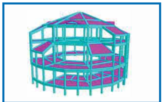
Fig. 7: 3D Analysis of Building considering Diaphragm Action of slabs – A diaphragm transmits lateral load to the vertical resisting elements
