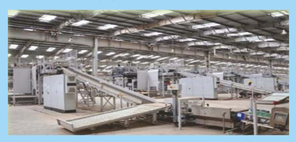
2 Engineering for procurement of Sulphur forming and handling system comprising of SS silos (6 nos. each of 550 MT capacity) conveying system and truck loading system with a Sulphur production capacity of 800 MT/day, largest ever handled in sulphur forming unit of IREP-BPCL-Kochi Refinery.
