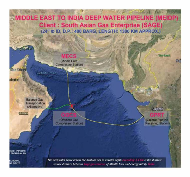
SAGE (South Asia Gas Enterprise Pvt. Ltd.) has been developing the deep sea offshore gas pipeline project from Middle East to India. The pipeline is anticipated to be the first of many in a corridor of pipelines that will form the final leg of a major energy supply route linking the Middle East with India. Middle East to India Deepwater Pipeline (MEIDP) offshore route traverses 1300
